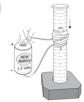
The coil will become an electro-magnet and the pin-ball will take a deep dive. On disconnecting the battery the pin-ball diver will pop up.
