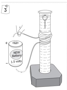
Scrape the insulation from the ends of the coil and attach them to a 1.5-volt battery.
