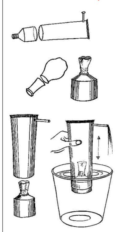
This pump is just like the Jerk Pump. The only difference is that the materials used, both for the pipe and the valve are very different.
