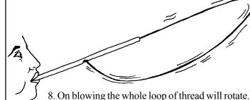
8. On blowing the whole loop of thread will rotate. Every fiber in the thread will get a push and the whole loop of thread will go round-and-round. If the knot gets stuck in the hole then either make the knot small or make the hole bigger.
