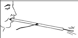
5. Take a 50-cm long piece of cotton thread. Place one end of the thread in this hole and gently blow from the other end to push the thread through.
