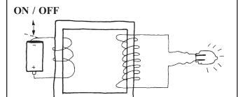
2. At this stage the 220-volt bulb will not light up. But as the battery contact is put ON / OFF the bulb lights up. We know that AC flows at 50 cycles/second. So by switching ON and OFF we are simulating an AC current.
