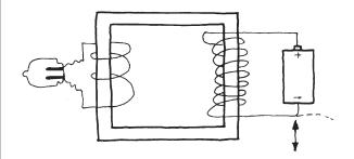
1. Normally electrical transformers works on AC. But you can make one work with a 1.5-volt DC torch battery. Take an ordinary transformer 220 volts to 3-volt (500 mA) used in many variable power supplies. Attach the Primary lead of the transformer to the battery. Attach the Secondary leads of the transformer to a 220-volt (25 W) ornamental / flickering bulb.
