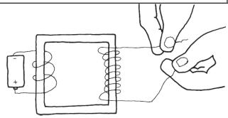
4. Now remove the bulb. Ask your friend to hold the two leads of the secondary coil with each hand. At this moment only one end of the battery is connected to the primary coil.
