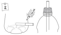
Press fit the short straw near the bottle base and the long one in the lid. Apply glue to prevent leakage.
