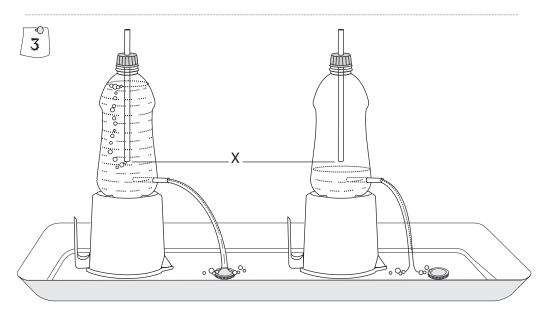
Place water filled bottle on a stand. Water will fall from the lower straw at a constant rate (on the COIN) until the "X" level. Below this level the water flow will reduce. This is because the air pressure at point "X" is the same as the air pressure outside.
