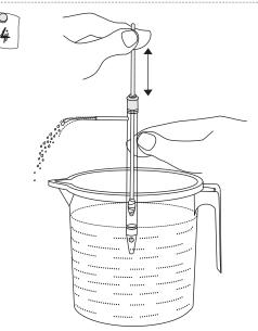
Place the Pen Pump in a mug of water and move the bicycle spoke-piston up and down. After a few strokes water will come out with a gush from the delivery pipe.
