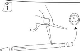
Make a hole in the end cap of an old pen so that a bicycle spoke can move freely in it. Make a small hole in the body of the ball pen for the delivery pipe.
