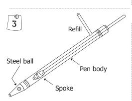
First drop the ball in the pen. Then insert the spoke-piston and finally screw the end cap. The refill should be inserted in the pen body in the end.
