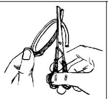
2. With a sharp scissors cut and remove the outer circle of the cap. The inner circle will make a superb piston. Rub it a little on sandpaper so that it is free inside the bottle - the cylinder.
