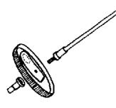
4. Cut a 12-cm long piece from a bicycle spoke Fix the piston on the spoke threads with two nipple nuts.
