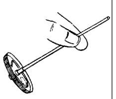
5. This is the piston, delivery valve and connecting rod assembly.
