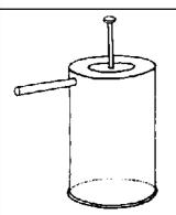
7. Make a 3-mm hole in the centre of the bottle base so that the cycle spoke can move freely in it. Make another hole on the curved surface near the base and fix an old refill or Frooti straw in it. This is the delivery pipe.
