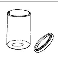
1. For making this pump you will require a black film-reel bottle, one more cap, a cycle spoke, old cycle tube, an old refill, simple hand tools and Fevibond - a rubber adhesive.
