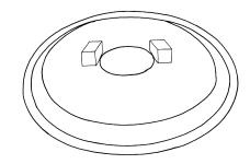
3. Fix two foam blocks diametrically opposite near the hole with adhesive.
