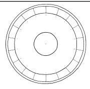
2. Cut a 7-cm hole in the centre of the foam plate.
