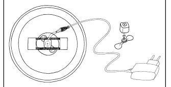
6. Mount the motor with the propellor on to the wooden slats. Attact the leads of the motor to a mobile charger which can be directly connected to a 220-volt power supply.
