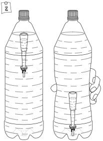
Place this "critically balanced" dropper in a 2-liter water bottle. Screw the lid tightly. On pressing the bottle a little water will enter the dropper making it slightly heavy. The dropper will dive to the bottom.
