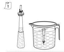
Place a cycle nut in a plastic dropper and tie it with a rubber band. Fill enough water in the dropper so that it just floats flush with the water level. The dropper will be critically balanced. It will neither pop out of water nor sink.
