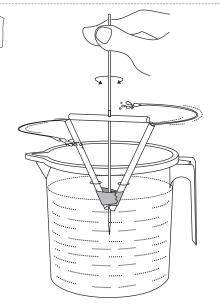
Place the triangle in water and spin the broom stick with one hand. Large chunks of water will sprinkle out from the straw cuts like a centrifuge.
