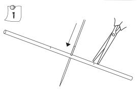
Poke the stick at right angles in the center of the straw. Mark two points 2-cm from the center and make half cuts.
