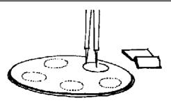
6. Cut two 10-cm. discs from card-sheet. Cut five circular windows in each disc with a divider.
