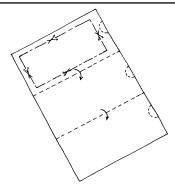
1. Take a card sheet 21-cm x 12-cm. Fold it into three. Cut out a window from the top rectangle. Cut semicircles on the right edge.
