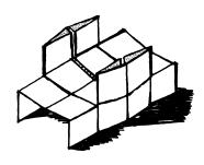
6. The assembly shows two 4 x 2 beds, placed side-by-side. The two 4 x 2 pieces have their folded doors facing each other.
