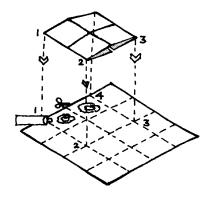
4. Take the other 4 x 4 square and cut it along the midline only up to the center point. Apply glue to the two little squares and stick one 4 x 2 piece as shown.
